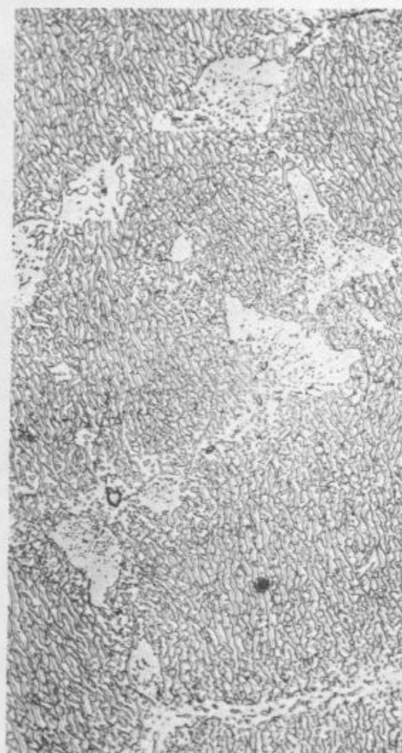
Coarse grain - 1800°F/942 hrs. 500X (b)
