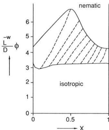
**Figure 3.** Volume fraction scaled by the weight-averaged length against mole fraction of the longer rods for a bidisperse mixture of rods ( $L_2/L_1 = 2$ ). The broken lines indicate in which two phases compositions falling in the two-phase region will divide.
