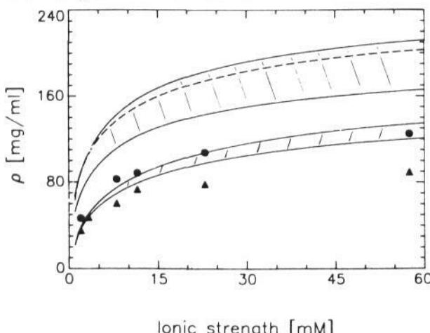
**Figure 10.** The concentrations of coexisting isotropic ( $\blacktriangle$ ) and nematic ( $\bullet$ ) phases of TMV at  $\text{pH} = 8.0$  plotted as a function of ionic strength. The calculated coexistence region is plotted for the second virial theory (negative-sloping hatching, see section 2.6) and the Parsons(-Lee) theory with an effective diameter (positive-sloping hatching, see section 3.3.4) (reproduced with permission from Fraden *et al* (1989)).
