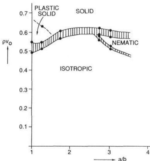
**Figure 5.** Phase diagram for prolate hard ellipsoids obtained by computer simulation (see text).
