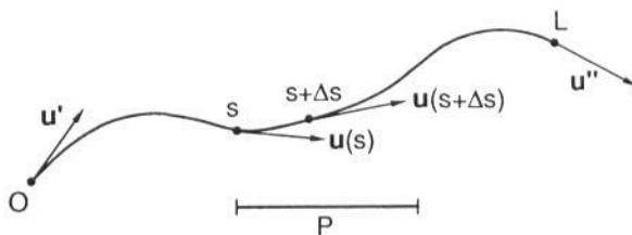
**Figure 8.** A typical configuration of a wormlike chain of length  $L$  and persistence length  $P$ .  $s$  measures the distance along the contour of the chain and  $\mathbf{u}(s)$  is the direction vector of the chain at this point.
