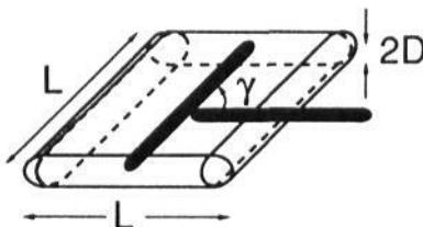
Figure 1. The excluded volume of two spherocylinders.
