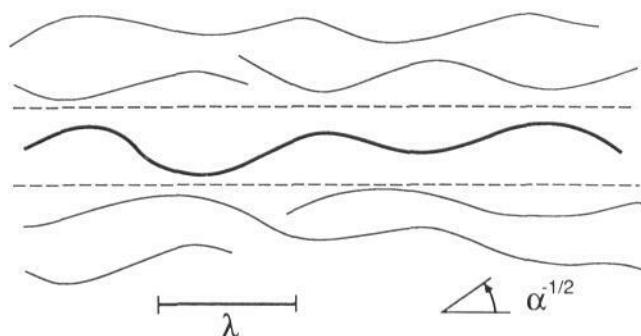
**Figure 9.** Each chain is confined by its neighbours to remain within an angle of about  $\alpha^{-1/2}$  from the (horizontal) director. Therefore the typical length scale of fluctuations is given by deflection length  $\lambda$  (see text).
