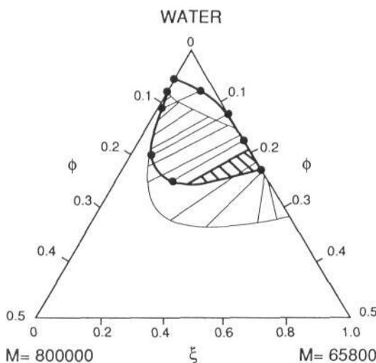
**Figure 13.** Ternary phase diagram for the system schizophylan ( $M = 800\,000$ )/ schizophylan ( $M = 65\,800$ )/ water: bold curves, experimental regions of phase separation (triphasic region indicated by negative-sloping hatching); thin curves, theory according to Odijk (1986a) (after Sato *et al.* (1989)).
