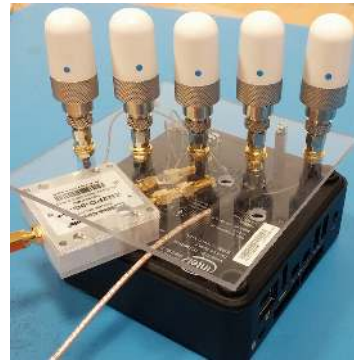
Figure 8: The 5-antenna Phaser AP with one antenna shared by both NICs. The signal from this shared antenna is split and fed into one RF front end on each NICs.
