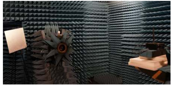
Figure 11: AP (far) and client (near) setup in anechoic chamber with multipath reflector.
