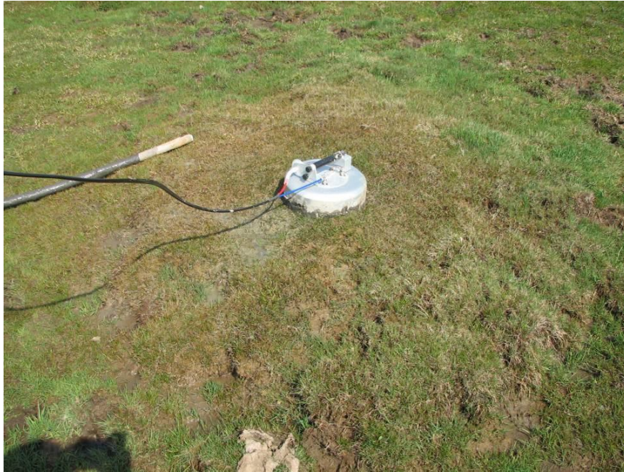
Fig. 6.4.3 Measurements in the area of mud zones with obvious soil vaulting /arched soil due to gas accumulations
