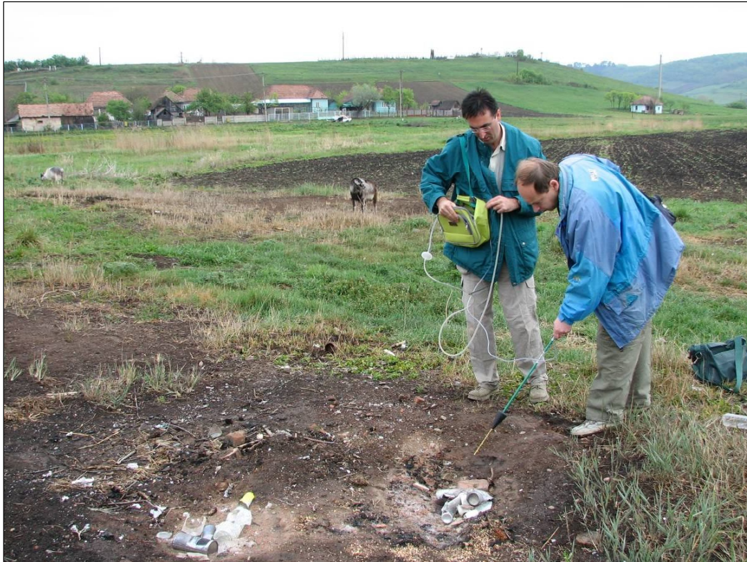
Fig. 6.2.3 Measurements of the methane flux in one of the chimneys of the Sărmășel everlasting fires, using METREX 2, Huberg, to record the methane values in air, close to the fires.
