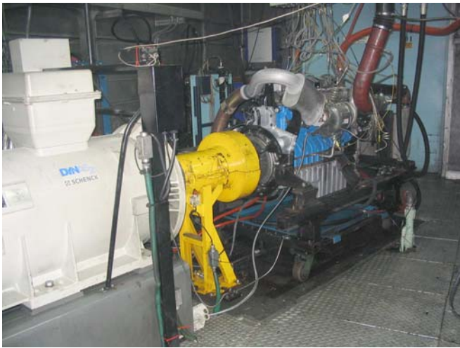
Figure 5. Six cylinder engine on DaimlerChrysler-Brazil test bench.
