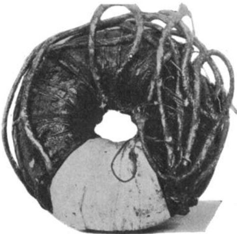
FIG 18—LOADING COIL WITH WINDING COMPLETED
