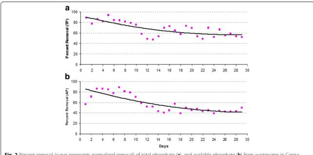
Fig. 2 Percent removal (curve represents normalized removal) of total phosphate (a), and available phosphate (b) from wastewater in Cannabased constructed wetland
