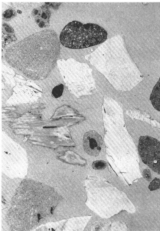
Figure 14. Photomicrograph of coarse grained P-phosphatic sand of Pliocene age. Note abundance of coarse fish debris and rounded, uncoated phosphatic peloids; Sample 112-680B-11H-1, 123-125 cm; scale bar is 1 mm.
