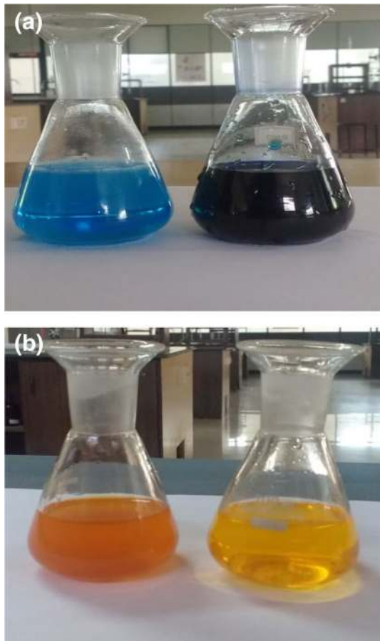
Fig. 10 a Degradation of MB onto CBMO before and after treatment. b Degradation of MO onto CBMO before and after treatment
