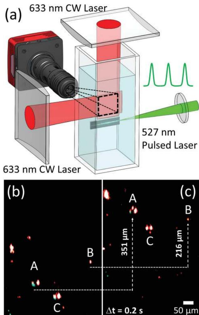
**Fig. 2** Experimental setup to observe and identify photothermal bubbles above the laser beam. (a) Experimental setup. A light sheet is created above the laser beam with a 633 nm laser. (b, c) Identification of bubbles from their shapes, large sizes and faster speeds moving to the water surface.
