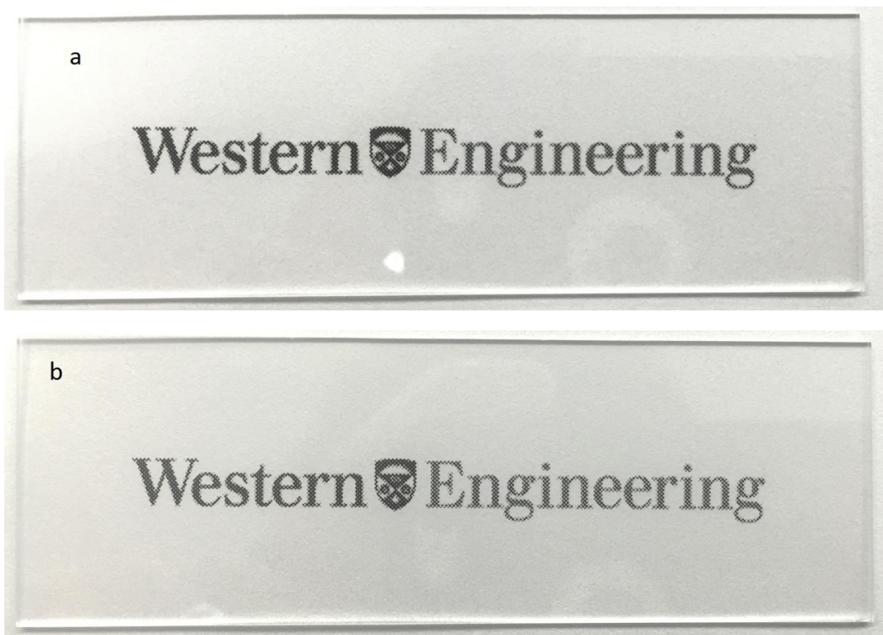
Figure 5.5. Photo of transparency of quartz plate (a) blank; (b) coated with polyurethane coating
