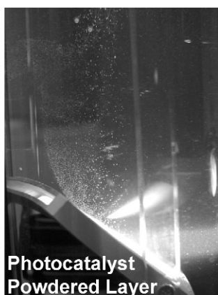
Fig. 6 Water splitting over NiO/NaTaO 3 :La photocatalyst under UV irradiation. Light source: 200-W Xe–Hg Lamp.
