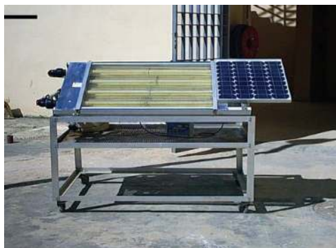
FIGURE 1: Photograph of the autonomous AQUACAT solar pilot prototype.
