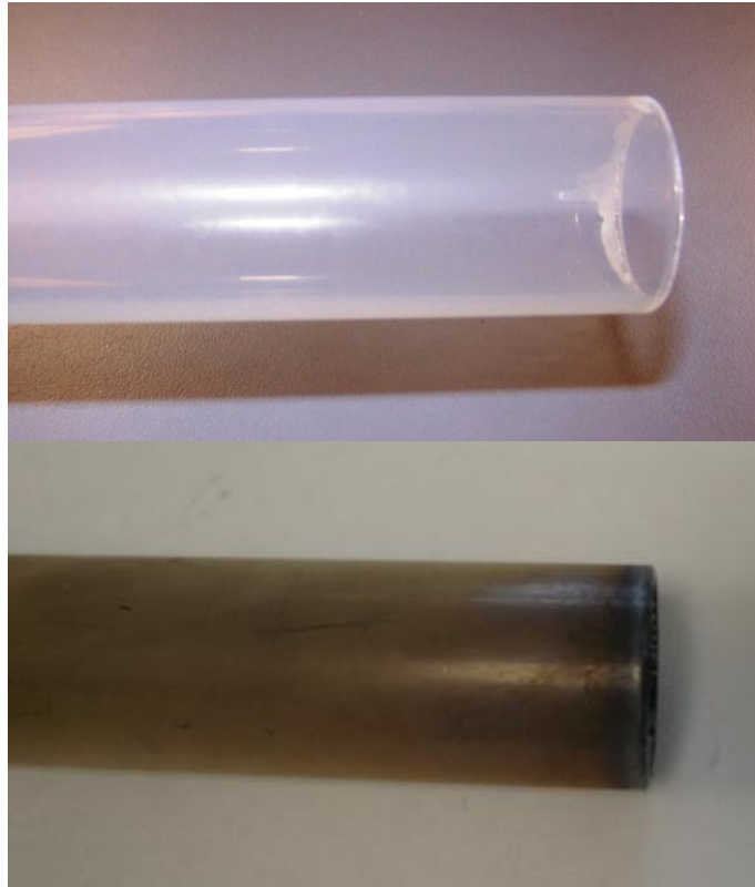
Figure 6. Photographs of the \text{TiO}_2 and \text{Ag/TiO}_2 photocatalytic wall systems.
