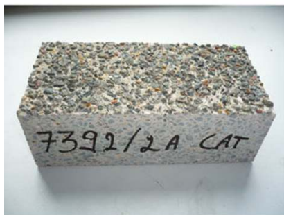
Fig. 14 Effect of different photocatalytic products (1=integrated in cement, 2=TiO 2 powder and 3=TiO 2 suspension) mixed in the mass of the concrete (no curing compound, modified curing procedure)
