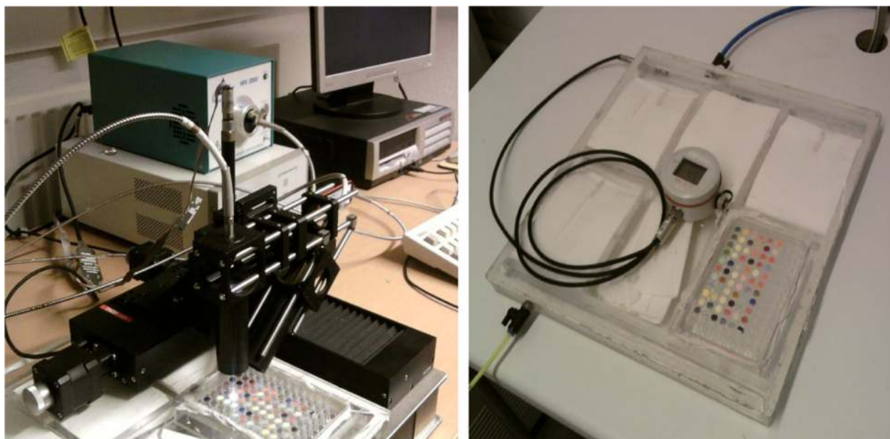
Figure 1 Left: The automated micro-fadometer system which controls movement of the probe head via the attached motorised XYZ stage. Right: a coloured set in the sample chamber.
