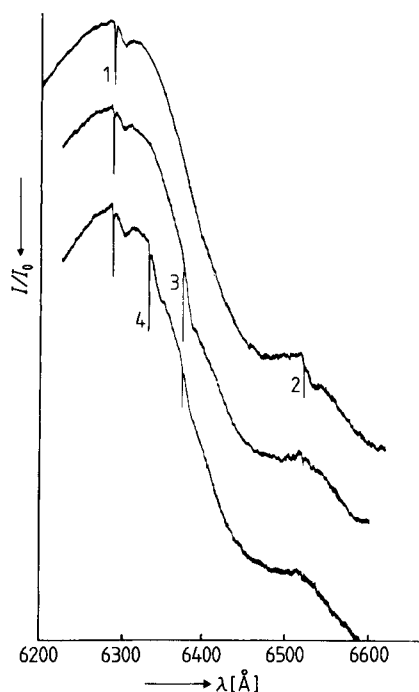
Fig. 38. Photochemical holes in the lowest energy band of phycocyanin + allophycocyanin. The numbers label the sequence of hole burning events [141]. T = 1.8 K, resolution 0.15 Å.
