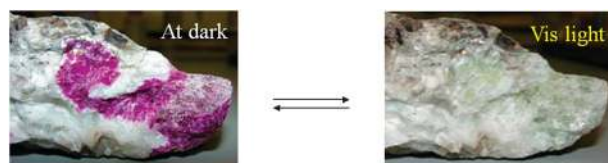
Fig. 2 Photochromic mineral (Hackmanite, \text{Na}_8\text{Al}_6\text{Si}_6\text{O}_{24}\text{Cl}_2 ) made by nature.
