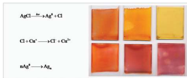
Fig. 3 Steps of the formation of the metallic silver particles upon irradiation and sol–gel photochromic coatings based on AgCl, after irradiation with UV light. Particle size ranging from 8 nm (yellow) to 30 nm (purple).
