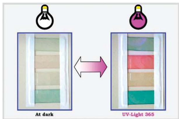
Fig. 12 Picture of the thin films prepared with different photochromic dyes, before and after irradiation with UV light.
