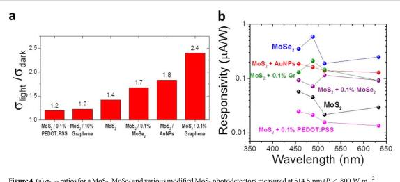
**Figure 4.** (a)  $\sigma_{\rm L/D}$  ratios for a MoS<sub>2</sub>, MoSe<sub>2</sub> and various modified MoS<sub>2</sub> photodetectors measured at 514.5 nm ( $P < 800~{\rm W~m}^{-2}$ ,  $V_{\rm b} = 1~{\rm V}$ ). (b) Responsivity for MoS<sub>2</sub>, MoSe<sub>2</sub> and various modified MoS<sub>2</sub> photodetectors as a function of the laser wavelength ( $P < 800~{\rm W~m}^{-2}$ ,  $V_{\rm b} = 1~{\rm V}$ ).
