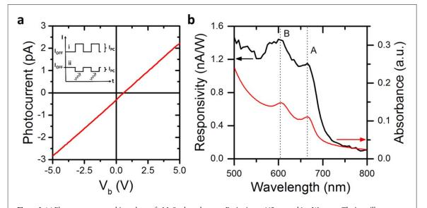
**Figure 3.** (a) Photocurrent versus bias voltage of a  $MoS_2$  photodetector. Excitation at 665 nm and 1 mW power. The inset illustrates the measurement scheme. (b) Responsivity as a function of wavelength (black line) for  $MoS_2$  at 4 V bias in comparison with the absorption spectrum (red line) of a  $MoS_2$  thin film of similar thickness. The dotted vertical lines mark the energetic positions of the A and B excitons at 665 nm and 606 nm, respectively.
