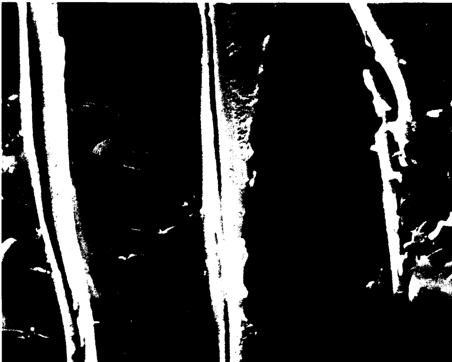
FIG. 7. Deterioration of half-bordered pits and cell wall of southern yellow pine at radial section after exposure to ultraviolet light for 500 h ( \times 1,000 ).
