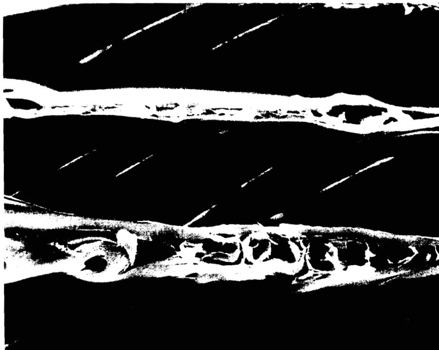
FIG. 9. Microchecks of cell wall of southern yellow pine at tangential section (earlywood) after exposure to ultraviolet light for 500 h ( \times 1,000 ).
