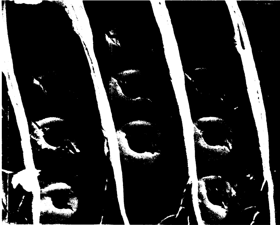
FIG. 14. Microchecks of cell wall of southern yellow pine treated with 10% chromic acid solution after exposure to ultraviolet light for 1,000 h ( \times 1,000 ).
