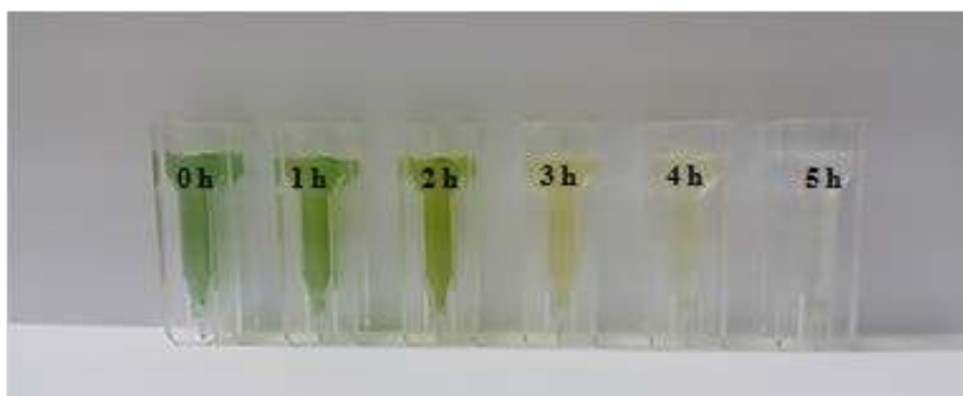
Figure 7. Photograph showing a change in the colour of binary dyes with increasing exposure time (0 - 5 h) to the UV lamp (365 nm) indicating that with increased exposure to UV light irradiation, the colour of the dye mixture steadily disappeared and finally the dye became nearly colourless.
