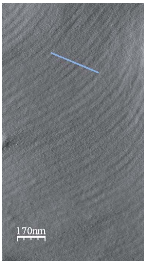
Fig. 18 Tapping mode AFM image of a homoepitaxial In-rich p-InP layer (see surface atomic arrangement in Fig. 16), showing atomic terraces with widths of about 50 nm.
