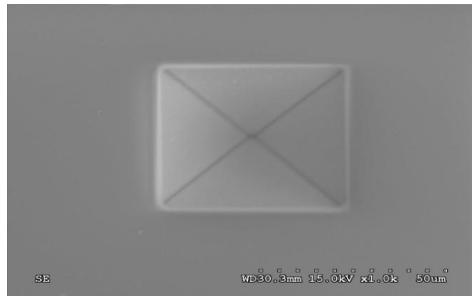
Figure 2.2. SEM image showing the top view of a KOH pit in Si (100).
