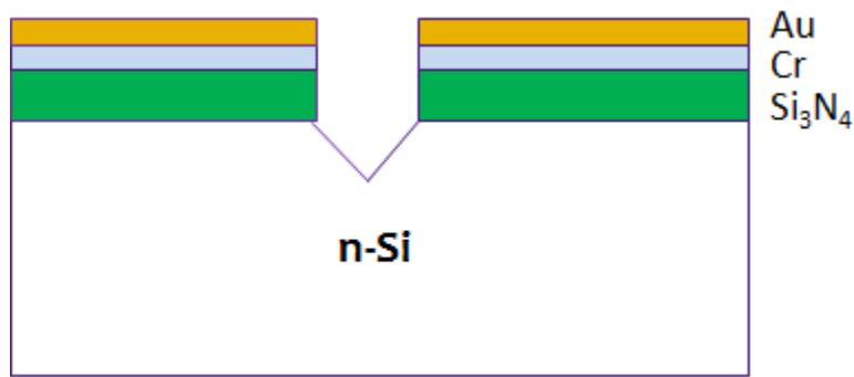
Figure 3.1. Patterned substrate for subsequent photo-electrochemical etching.
