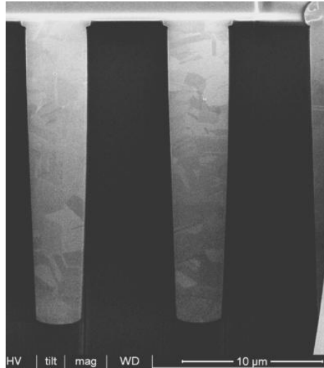
Figure 1.2. Copper filled TSVs. Reference Van Olmen et al., “3D Stacked IC Demonstration using a Through Silicon Via First Approach”, IEEE Conference Proceedings publication (© 2008 IEEE).
