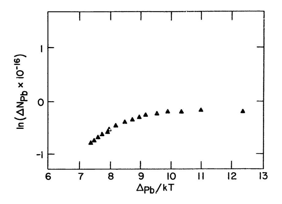
curve  $\Delta N_{exp}^{Pb}$  versus  $\Delta_{Pb}/kT$  for the same value of  $\varepsilon^*$ . It can be seen that the lead curve shows saturation.
