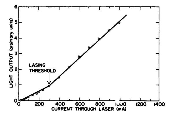
in the derivative of the light output versus current at the lasing threshold decreases) after several months of use. This is possibly due to thermal recycling and self-induced damage due to heating.
