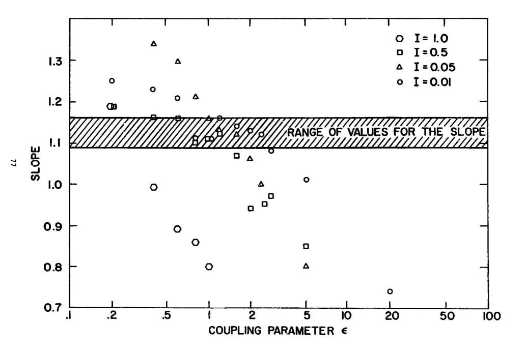
Fig. IV-11. Slopes of  $\ln(\Delta N_{Sn})$  versus  $\Delta_{Sn}/kT$  plotted as a function of the coupling parameter  $\varepsilon'$  for the case when Sn is illuminated for different relative illuminations. The dashed area indicates the theoretical values of the slopes for low reduced temperatures. (For this graph  $\Delta N_{Sn}$  was determined using unenhanced densities of state.)
