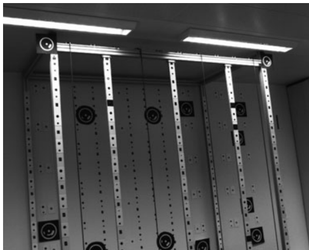
FIG. 8. The photogrammetric 3D calibration field at the Institute of Geodesy and Photogrammetry at ETH Zurich. The picture was taken by CAM1.
