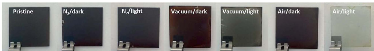
Fig. 1 Photographs of \text{CH}_3\text{NH}_3\text{PbI}_3 films exposed in several atmospheres for 24 hours.
