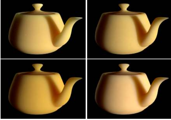
Figure 8: Comparison between volumetric path-tracing (top left), our method (top right), our method with multiple scattering only (bottom left), and dipole diffusion (bottom right). The dipole produces color shifts and over-smoothing due to an inaccurate profile. (Parameters: \sigma'_s = 1, \sigma_a = (0.01, 0.1, 1), \eta = 1, g = 0 .)
