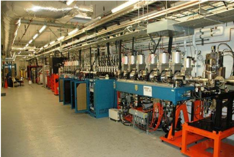
Fig. 2: Downstream view of the FEE. From the right: Slit system, attenuator system, total energy monitor (black cube) and the mirror system in the background.
