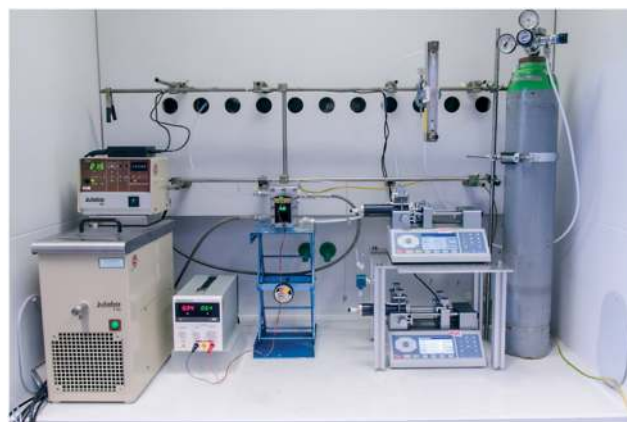
Fig. 2 Lab plant used for photochemical transformations with a falling film microreactor as core element.
