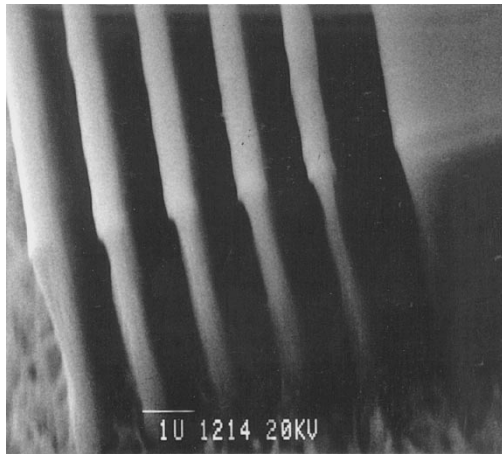
Fig. 5. Ultra-deep 3\lambda_s/4n grating formed into InP substrate by \text{Cl}_2 RIBE.
