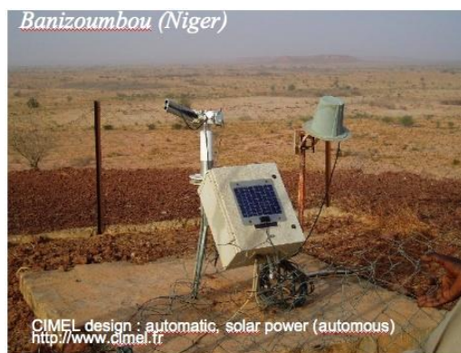
Fig. 2. Example of sunphotometer setup, in Africa.
