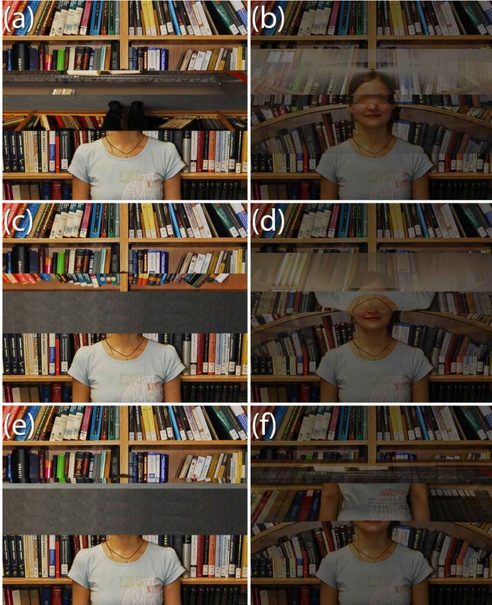
Fig. 3. The piecewise homogeneous positive uniaxial birefringent unidirectional free-space cloak under views away from the transformation axis. The bare mirror structure is shown and the corresponding cloaking result for horizontally linear polarized light, respectively for rotations of (a), (b) 5 degrees, (c), (d) 10 degrees, and (e), (f) 20 degrees around the axis of the cloak. The behavior of the unidirectional cloak for views not along the transformation axis is akin to a carpet cloak. Note the total internal reflection (TIR) in air at the first air-cloak for ordinary light interface due to \mu_o = 0.31 \ll 1 in the corresponding cloak segment.
