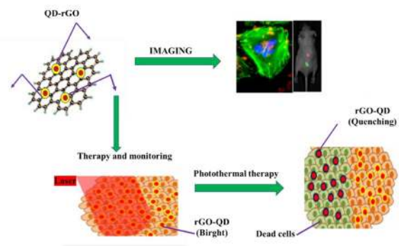
Fig. 4. rGO nanocomposites tagged with quantum dot (left) entered into targeted cancerous cells emit bright fluorescence from the quantum dots, (right); the absorption of NIR radiation by rGO and its conversion into heat, causing fluorescence reduction and cell death (Reproduced with permission [29]).
