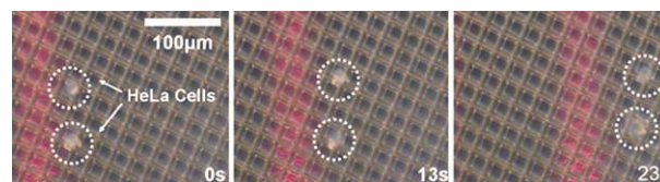
Fig. 7 Images of cells transported across the field of view. A line-shaped optical pattern pushed the HeLa cells as it scans from left to right. Each pixelated phototransistor has an area of 20 μm × 20 μm, with 2 μm isolation gaps. The applied voltage was 20 V pp . The grid background pattern is the phototransistor arrays; the red vertical line is the optical pattern.
