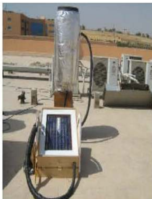
Fig. 2 Thermosyphon effect used on PV/T system, [15]
