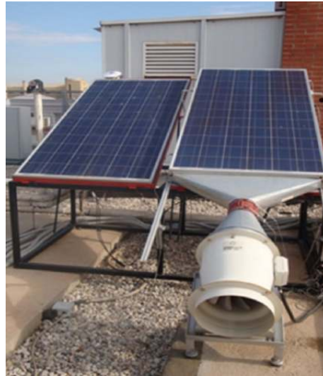
Fig. 4 Forced air cooling [10]
