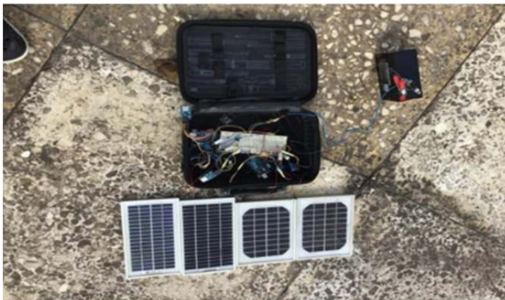
Figure 3: Experimental set-up of sprayed and unsprayed PV panel
