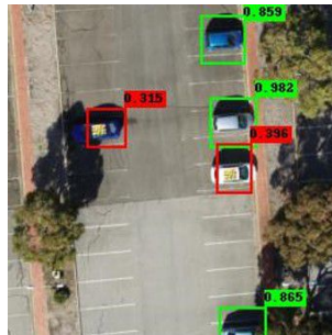
(e) Two of the cars from (c) imaged with physical on-car patches; their objectness scores reduced to 0.315 and 0.396.
