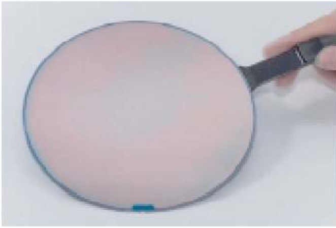
Fig. 18. Features of GeOI using epitaxial Ge on Si. (a) Top view photograph of a final GeOI wafer 200 mm in diameter ( T_{Ge} = 60 nm, T_{BOx} = 400 nm). The donor wafer is a 200 mm epiwafer [113]. (b) SIMS depth profile of the Si and Ge atoms inside a 2.5 \mu\text{m} thick Ge layer grown on Si(001) that has subsequently submitted to in situ anneals.
