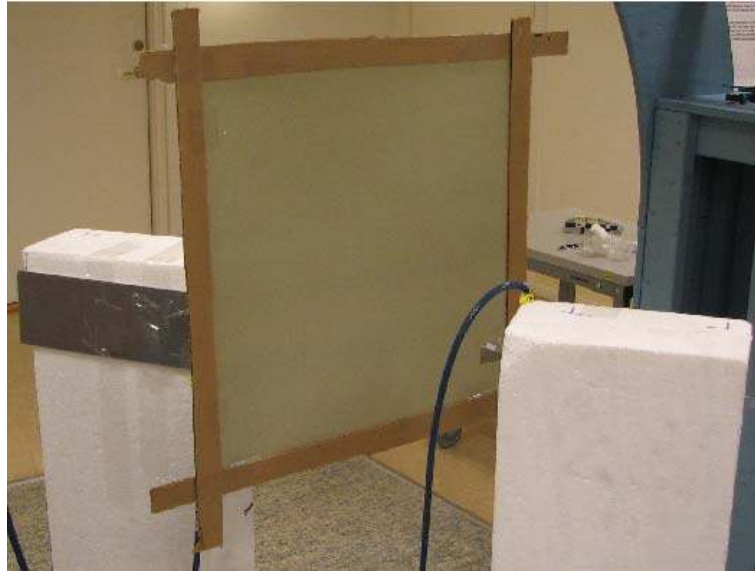
Figure 4: Measurement setup for oblique incidence on an array of split ring resonators. The sheet was oriented with the gaps in the split rings along the vertical direction.
