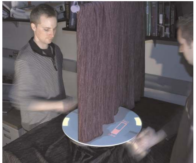
Fig. 1. Experimental setup with a two-handled crank. Two participants cooperate to complete a timed target acquisition task. They cannot see each other and are instructed not to speak, thus communication is limited to forces and motions transmitted through the rigid handles of the device. Picture digitally modified for clarity.
