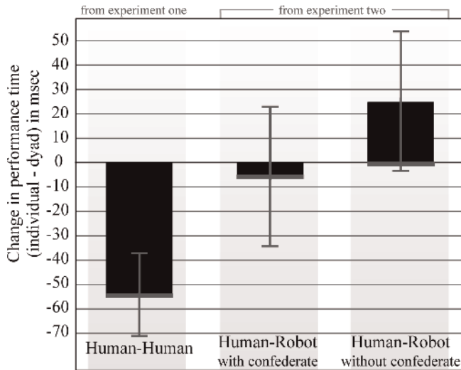
Fig. 6. Change in completion times. We programmed a robotic partner to simulate an acceleration specialized partner and compared the improvement time. Participants in the HRC group (middle) knew they were working with a robotic agent while participants in the HR group (right) believed they were working with a human but actually were not. Each dyad time is compared to the participant's individual time (normalized to 0), so a negative value means the two people (or human-robot pair) worked faster together than the individual. Two humans working together (left) were significantly faster than an individual working alone. When working with the robotic partner, participants with a confederate present are faster than participants without a confederate present. Error bars represent 95 percent confidence intervals.
