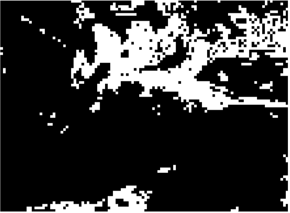
Figure 12. Cloud mask used for GOES-K retrievals. White regions designate detected clouds with stable ( \Delta - T_{10.7}(t_1, t_2) < 2.0^\circ\text{K} ) thermal background fields and zero-visible radiance at time t_2 (1730 Z, at time of total solar eclipse).
