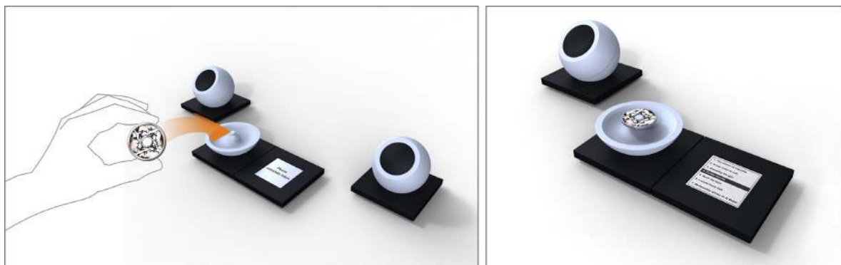
Figure 7. Left: The token is placed on the music player. Right: The music player in action.
