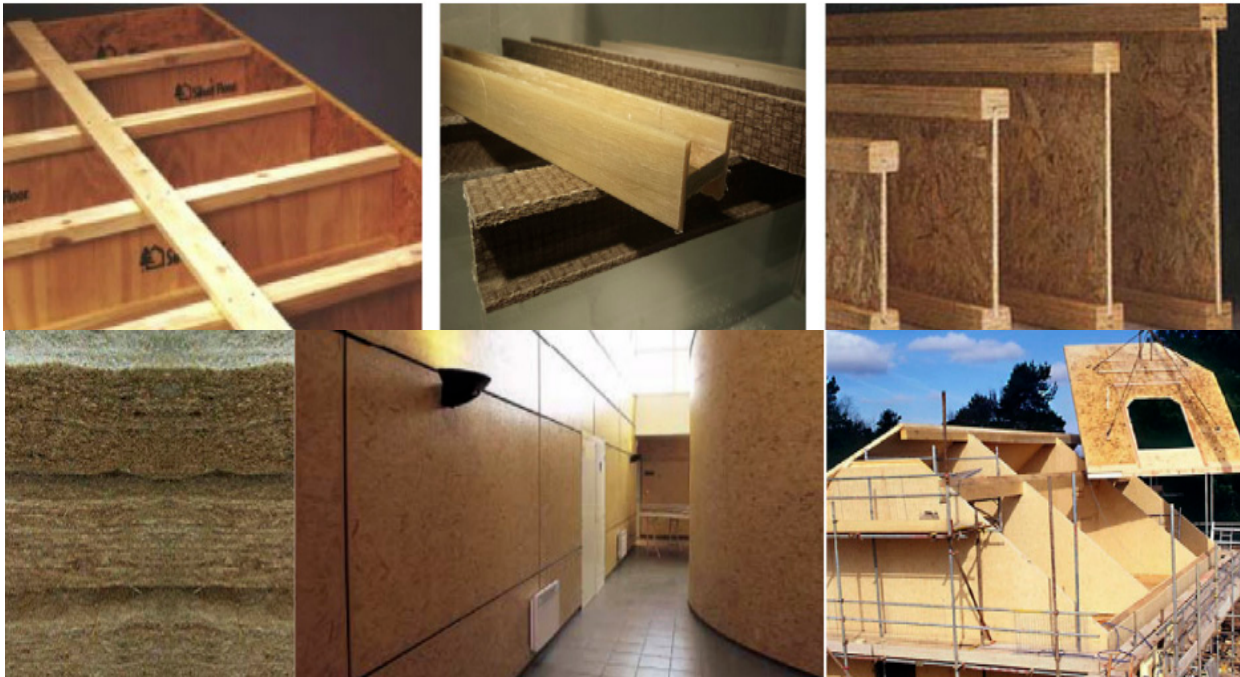
Figure 6. Construction components made NFRCs [181]. Reprinted with permission. Copyright 2020 Elsevier.
