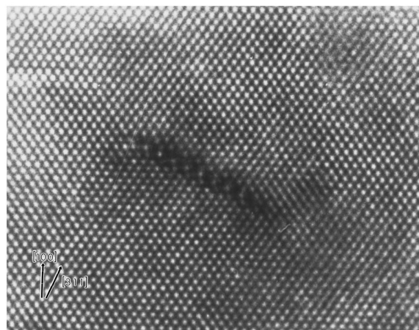
FIG. 2. Cross-section high-resolution electron micrograph showing \{311\} habit plane, and typical image contrast of \{311\} defects.
