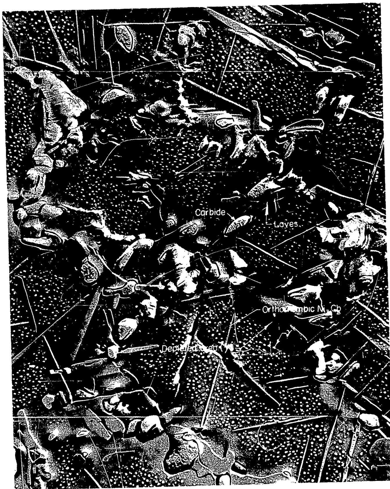
FIGURE 40. ALLOY 718 STRESS-RUPTURE SPECIMEN TESTED AT 1350 F, 10,000-PSI STRESS FOR 5470.7 HR (6) (Heat treatment: annealed at 1700 F, 1 hr, water quenched; aged at 1325 F, 16 hr, air cooled. Reduced approximately 20 percent in printing.)
