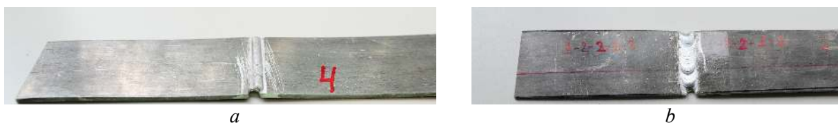
Fig. 5. Type of strip from the side of the weld (a) and back side (b)
