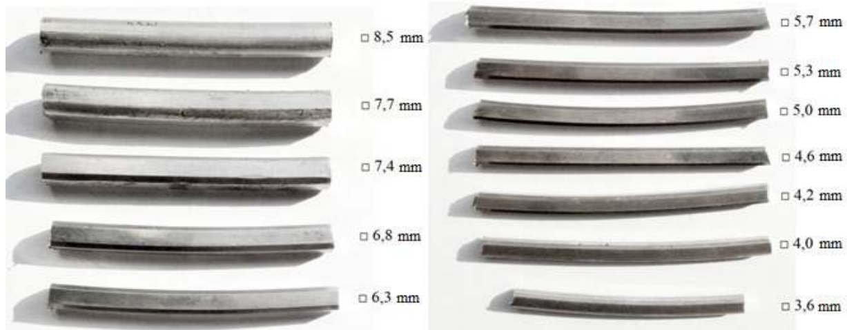
Fig. 4. Appearance of profiled rods after rolling
