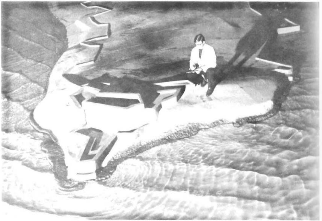
Figure 7. Three-dimensional wave action model of existing conditions at El Morro Castle.
