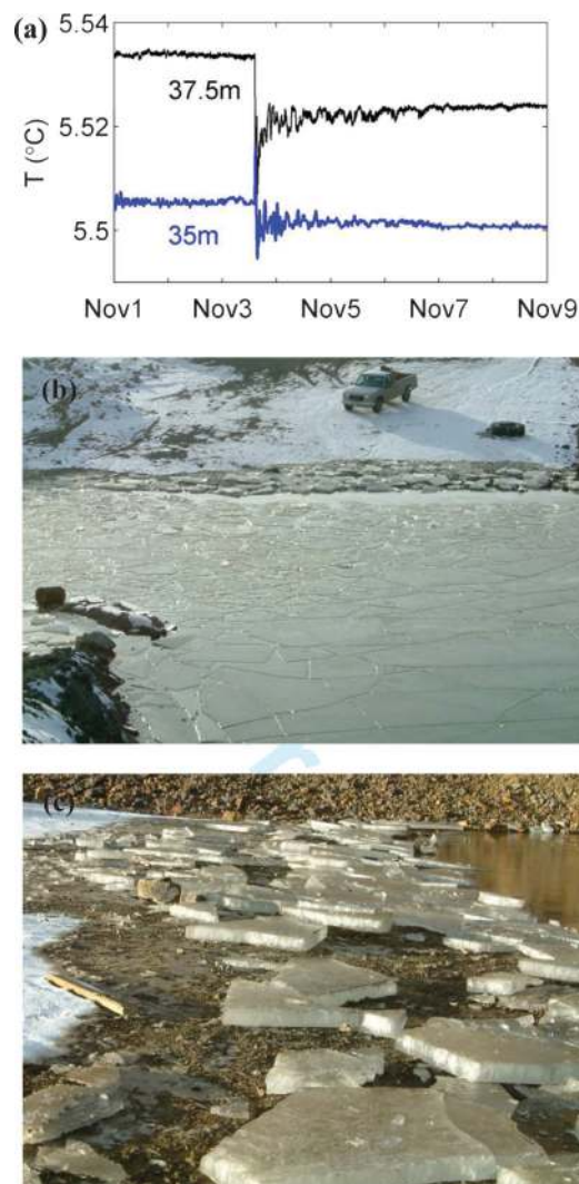
Fig. 10. The Alaska earthquake of 3 November 2001 (magnitude 7.9) as observed in the Waterline pit-lake. (a) Temperature at 35 and 37.5 m; note the temperature increases with depth, see Fig. 5a. (b), (c) Broken and dislodged ice cover after the earthquake. The temperature observations show that the earthquake generated internal seicheing and some mixing. Waterline is located 1600 km to the southeast of the earthquake epicenter. Photos courtesy of M. Aziz.
