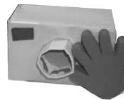
Figure 6: A large stuffed "hand" sensor that was placed on a child-created camera. When the hand was placed on the camera it could be physically programmed to be "touch sensitive". Therefore if a child touched the camera, a video might appear on the wall with a picture from the camera.
