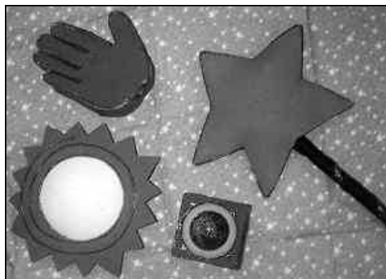
Figure 7: Physical icons for programming a StoryRoom; From left to right: A "hand" to make an object touch-sensitive; a "light" to make an object "light up"; a "sound box" to attach a sound to an object; a "magic wand" to signal the authoring mode.
