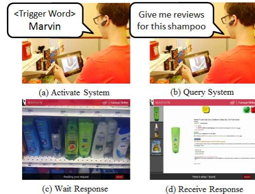
Figure 1. The use case: A person holding his mobile device toward the object of interest (a) activates the system via a trigger word, (b) makes a verbal query about the object, (c) waits for a response, and (d) receives the response on his display.
